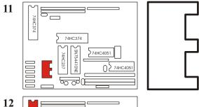
Solder in the battery connector into the spot labeled J7. Look at the shape of the connector, and make sure it matches the outline on the board, magnified to the left. **Make sure you orient it correctly!**
