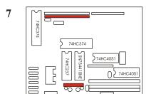
Cut a 14-pin section of **female** header and put it in location J1: it is your LCD connector. Use a remaining 6-pin section of female header as your motor connector in location J23 and J24. Keep them perpendicular to the PCB.
