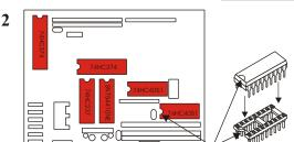
Carefully plug each of the ICs into its corresponding socket. The part numbers are printed on the board. The large board drawing on the first page of these instructions also has the IC locations labeled. Also, make sure the notched end of the IC matches up with the notches in the drawings.
