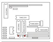
Bend the 330-ohm resistors into inverted "U" shapes as shown to the left, and solder into the locations labeled R5 and R6.
